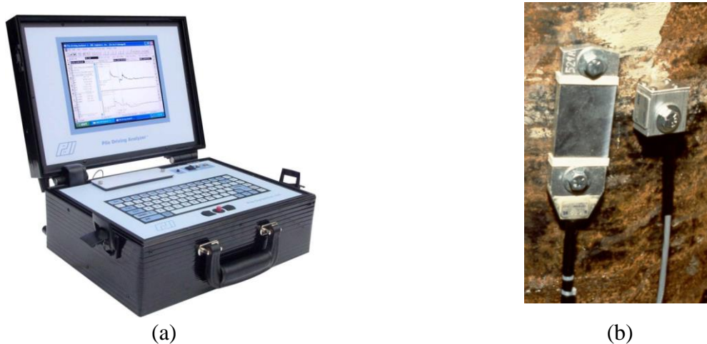
Figure 2-17 A typical PDA-system Consisting of (a) PDA-data Acquisition System and (b) a Pair of Strain Transducers and Accelerometers Bolted to Pile (Rausche, Nagy, Webster, & Liang, 2009).
